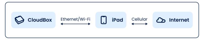
The iPad can communicate with the internet through cellular. The iPad will then communicate with the CloudBox over Wi-Fi or ethernet. FuelCloud recommends connecting the iPad directly to the CloudBox with the included ethernet cable.
