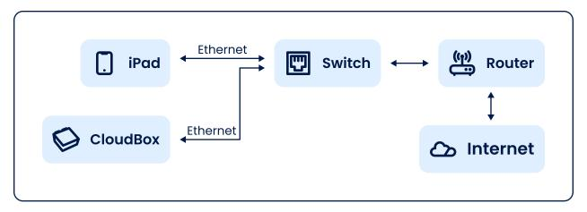
Connect the iPad, CloudBox, and router to an ethernet switch. If you did not purchase an optional ethernet switch, connect both directly to the router.
